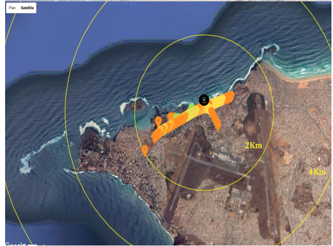
Fig. 9. Received RSSI from “Virage” Base Station.
