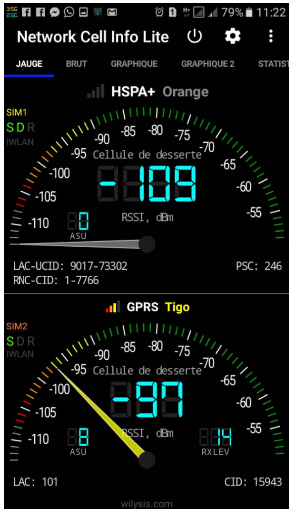
FIGURE 15 – 2G RSSI with Network Cell Info Lite application
