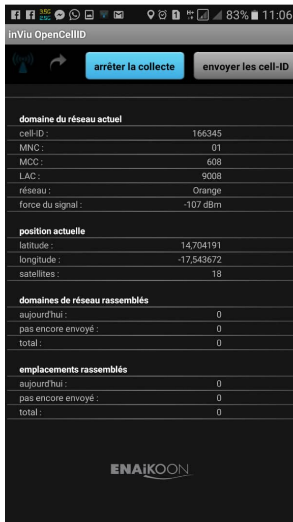
FIGURE 14 – 2G RSSI with “inViu OpenCellID” application
